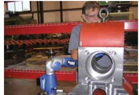
The FARO Gage is a portable CMM that was designed to enable machinists to speed through measurement challenges and produce the most accurate results possible. It allows measurements to be taken right on the shop floor, without the need of stopping production. The Gage provides excellent accuracy and because it offers portability and quick set up, it reduces inspection time. And since the Gage can automatically record measurements, inspection reports are easily generated.
