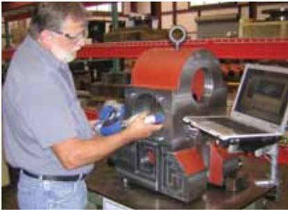
One of the many challenging projects that Ansko took on was the machining of a cast iron housing that weighs about 750 pounds. This part was too large and cumbersome to be inspected by Ansko's traditional bridge-type CMM.
